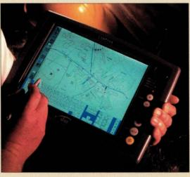
a complimentary hardware solution, J-Slate-a notepad-size, battery-powered diskless pen computer equipped with a 10.4-inch screen and touch-screen capabilities. The client software, running
