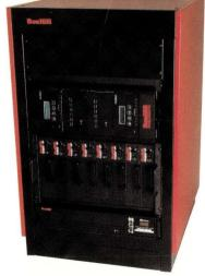
is simply a SMARTER hotswappable, modular RAID system with dual failover controllers.
